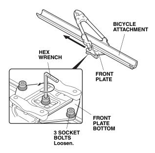
Set the front plate 245 mm (9.6 in.) from the end of the bicycle attachment, and retighten the three socket bolts on the bottom. Torque the three socket bolts to 8 N·m (5.9 lbf·ft). Rotate the arm as shown.
