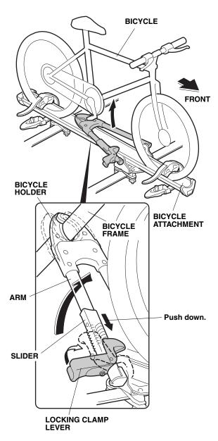
13. Push up the locking clamp lever to secure the bicycle frame.
